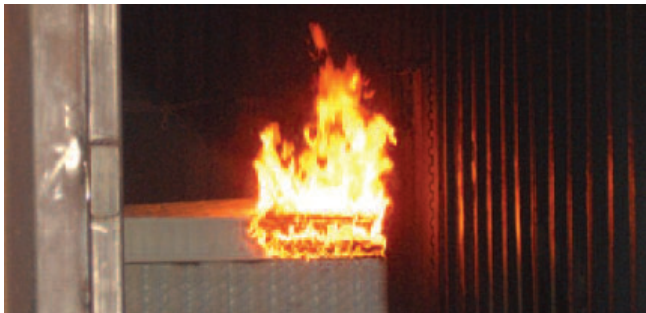
Flammability test of a non-conforming mattress – how safe are the products you buy?
